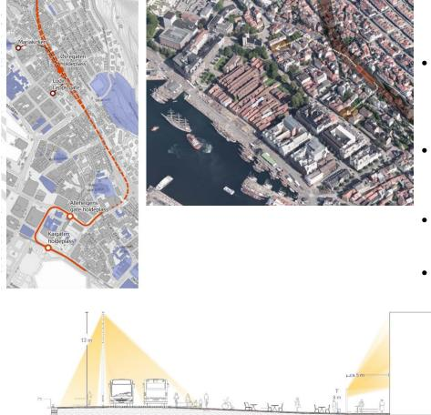
*Tunnel option: Systematic section shows concepts for lighting of planned bus track and cycle path (@Mijøløftet)*
